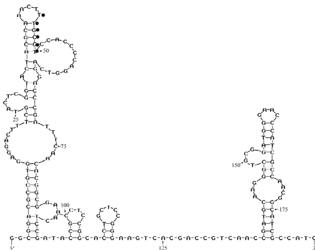
Fig. 3 Predicted secondary structure of the sso of pXT107
